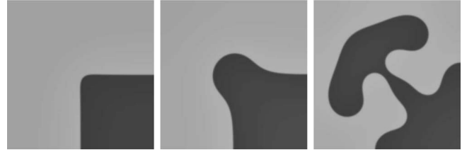
FIG. 10. Instability of the boundary. We show successive snapshots of a 2000 \times 2000 array with \Delta r=0.02 at t=0 , t=170 , and t=705 . The pattern slowly evolves throughout the whole space. a=1.475 .
